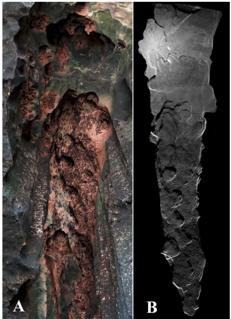
Fig. 2. A) Color photograph of the Swiftlet Slit, and B) TLS point cloud depiction of the same area. Note that the point-cloud provides a true planar view, without perspective distortion. View is vertically upwards, northwest at the top of the figure.
